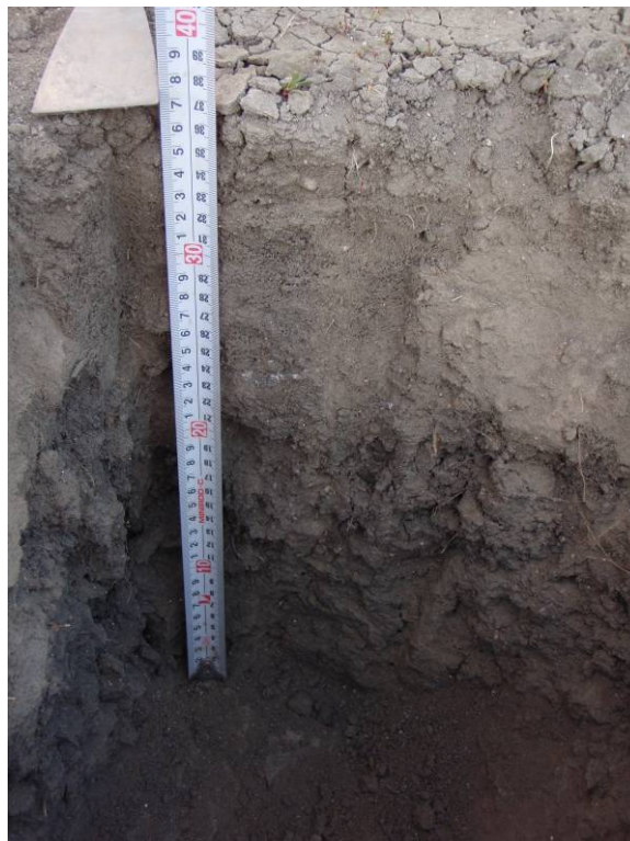
Figure 1-3 Typical grey clay soil profile in the Narran Lake Nature Reserve Ramsar wetlands (RSNL 19).
