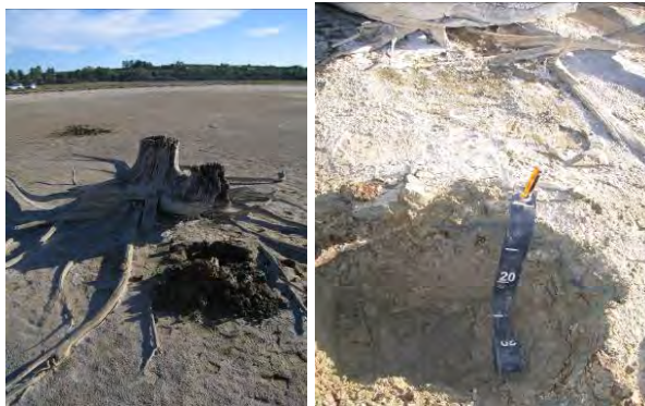
Figure 8-9. Photographs of Site 7, showing the site location next to a dead tree stump and the soil pit with salt crust on the soil surface.
