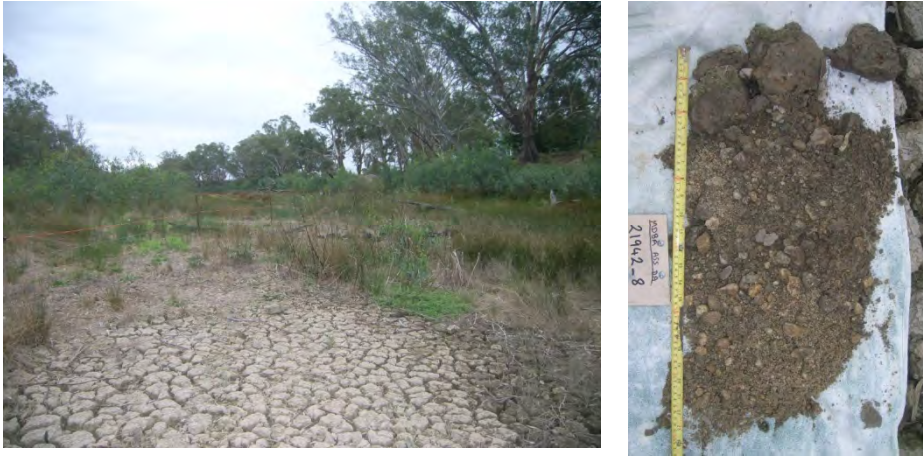
Figure 8-36. Photographs of site 21942_8, showing the bare cracking clay surface in the centre of the channel, and the soil profile.
