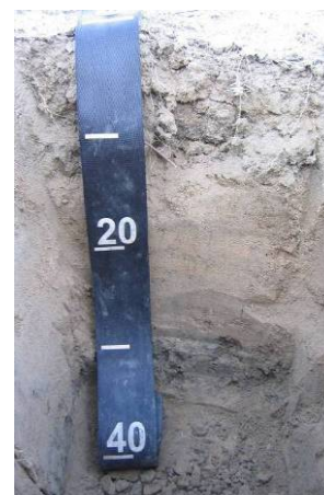
Figure 78-3. Photographs of the soil profile BFT2, showing the wetland margin at a high elevation, and the soil profile of friable, sandy loam to approximately 25 centimetres over very firm clay.
