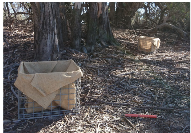
FIGURE 2 Litter trap used to estimate litter fall rates. The traps were steel mesh boxes ( 560 \times 450 \text{ mm} = 0.25 \text{ m}^2 ) with an open top, that were lined with hessian to retain organic material
