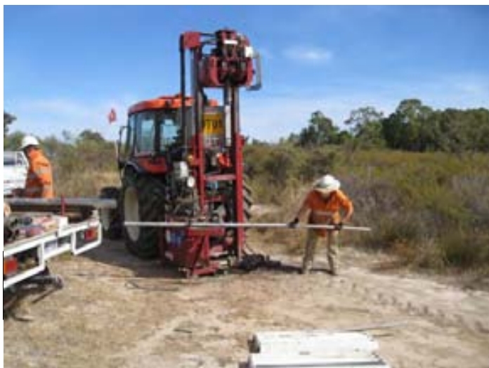
Sonic drilling rig used in the DEC Swan Coastal Plain ASS mapping program
