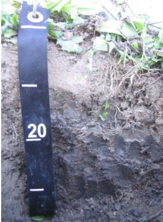
Figure 38-2. Photograph of site YHD1, showing the soil profile of black, rigid clay.
