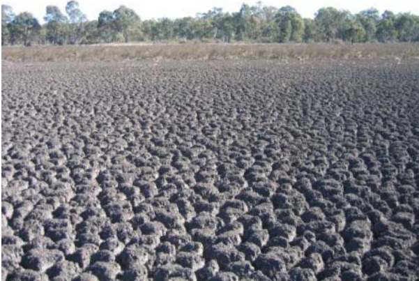
Figure 35-2: Photographs of site YHW1, showing the degrading bare cracking clay surface, and the soil profile of black rigid clay.
