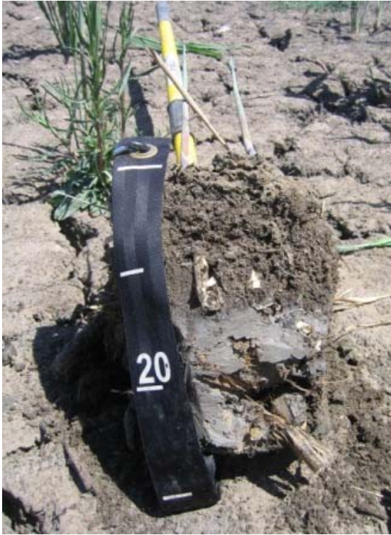
Figure 32-6. Photograph of site MSP5, showing the soil profile upper clay soil layers and the cracking clay surface.
