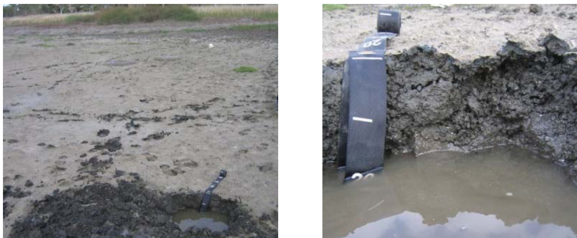
Figure 32-2. Photographs of site MSP1, showing the site location where the surface was a soft clay, and the soil profile with the water table at approximately 15 cm.
