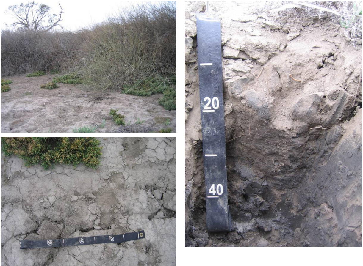
Figure 34-3. Photographs of site KIA2, showing the soft surface, adjacent to the Muehlenbeckia florulenta (Lignum) on the wetland margin, and the soil profile of hard, blocky structured, clay.
