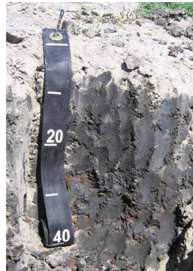
Figure 36-6. Photographs of site PFT5, showing the inlet channel, and the soil profile of black, extremely hard clay with red mottles in the matrix.
