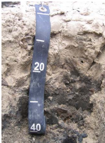
Figure 44-4. Photograph of site BWH3, showing the soil profile of the encroaching surface sand over very firm clay.
