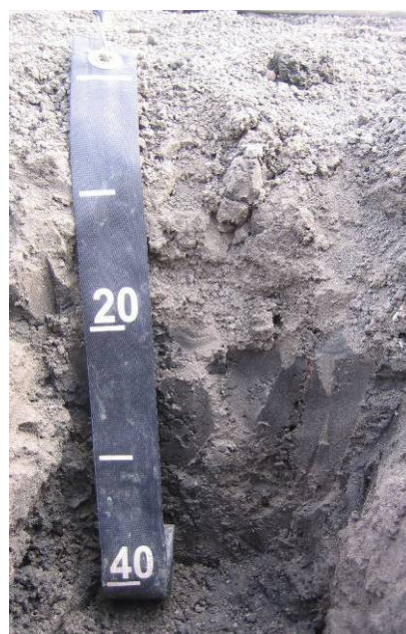
Figure 49-2. Photographs of site NCT1, showing the site location where the surface was bare, and the soil profile of black, slightly rigid, clay.
