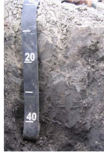
Figure 54-2. Photographs of site FRL1, showing the cracking clay surface of the main wetland area, and the soil profile of very firm clay.
