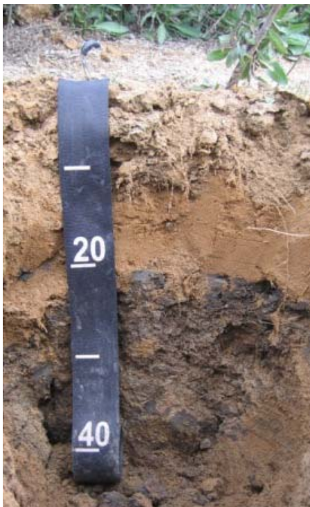
Figure 47-3. Photograph of profile CMT2, showing the soil profile with loose sand to about 15 cm over the grey clay.
