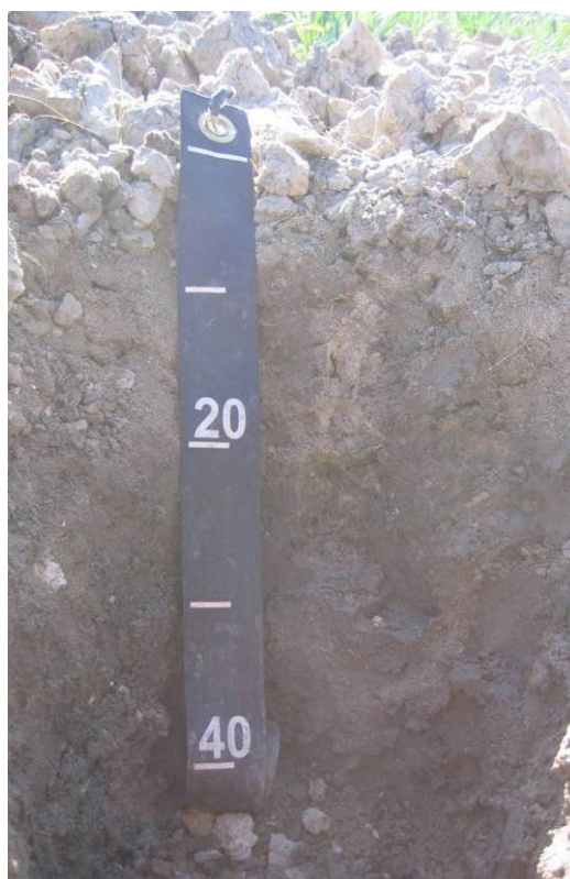
Figure 43-2. Photographs of site MDT1, showing the cultivated cloddy surface of the main wetland area, and the soil profile of rigid, cloddy, clay over very firm, clay.
