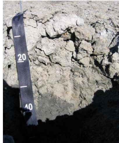
Figure 55-2. Photographs of site WON1, showing the main wetland area of cracking clay soils, and the soil profile of very firm clay.
