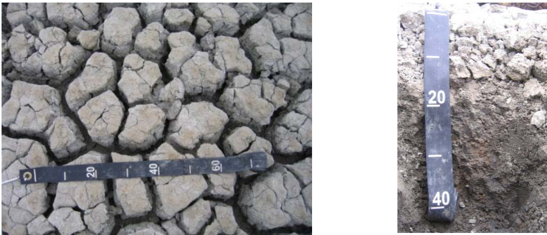
Figure 44-3. Photographs of site BWH2, showing the very hard clay surface with deep cracks, and the soil profile with a surface layer of extremely hard clay aggregates over a very firm clay.
