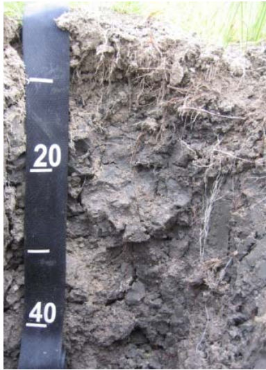
Figure 46-2. Photograph of site SBF1, showing the soil profile of a well structured firm clay soil.
