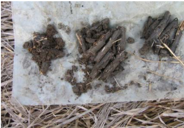
Figure 46-4. Photograph of site SBF3, showing the soil profile core with upper soil of brown friable clay on the left and grey firm clay on the right.
