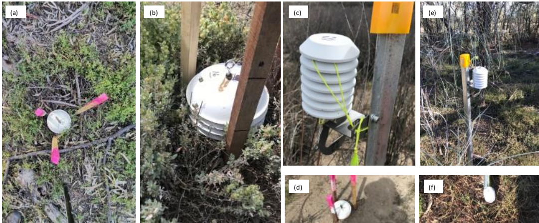
Figure 4 Photos (from left to right) showing the temperature and humidity sensors installed at (a) the River Red Gum understorey; (b) the Copperburr; and (c)-(d) two levels at the Lignum; and (e)-(f) two levels in the Black Box understorey site.
