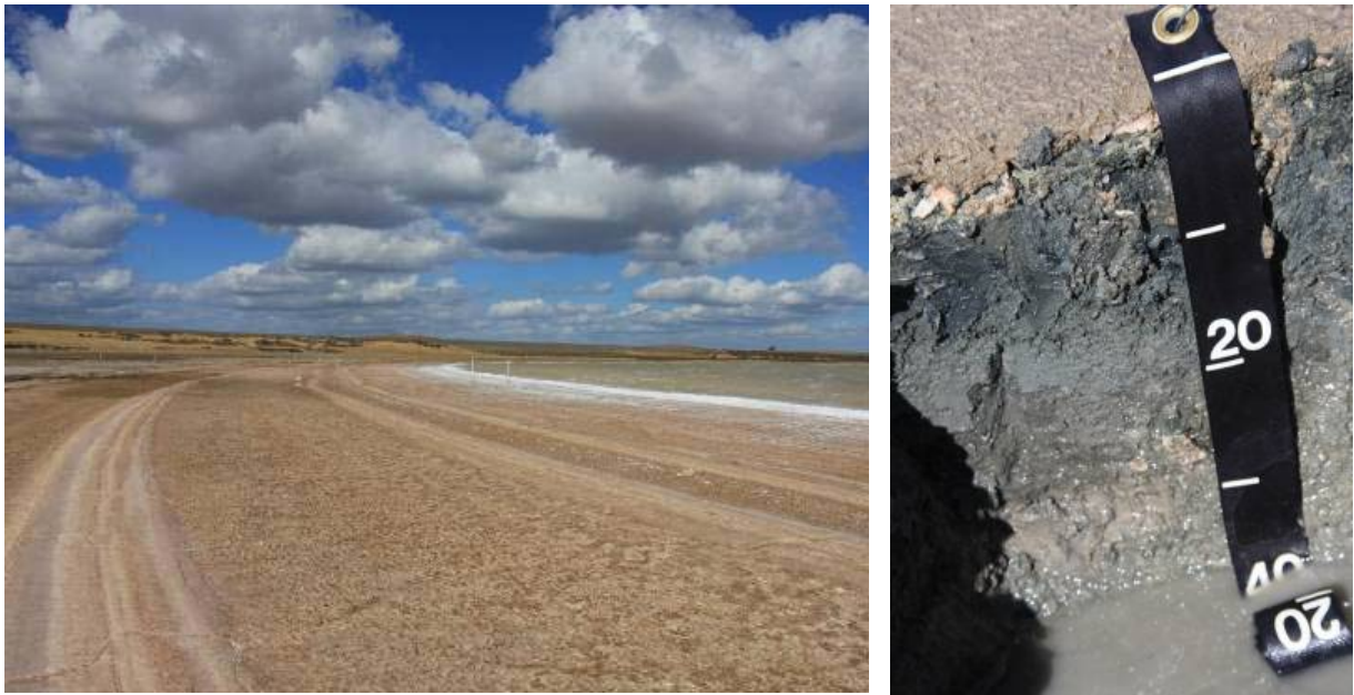
Figure 2-2 (left) Landscape photo of Lake William (sites KER 21 and KER 22), a hypersaline lake with the shore encrusted with windblown salt up to 20 cm thick. (right) Soil profile KER 22 sampled from near the waterline. Dark grey to black layers indicate the presence of monosulfidic material.
