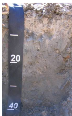
Figure 62-3. Photograph of the soil profile PRE2, showing the soft clay soil.
