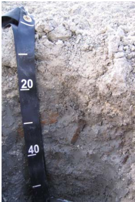
Figure 66-2. Photograph of site MLA1, showing the soil profile of friable surface aggregates and a firm subsoil clay.
