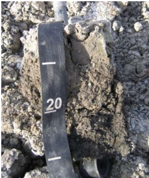
Figure 66-6. Photograph of site MLG5, showing the soil profile of the upper soil layers of friable aggregated clay.
