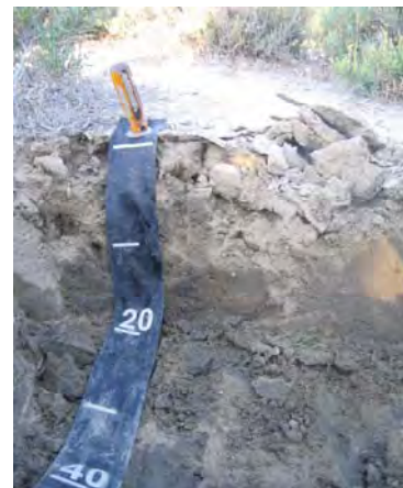
Figure 9-6. Photograph of Site 18, showing the soil profile with a sealed surface containing salt efflorescences.
