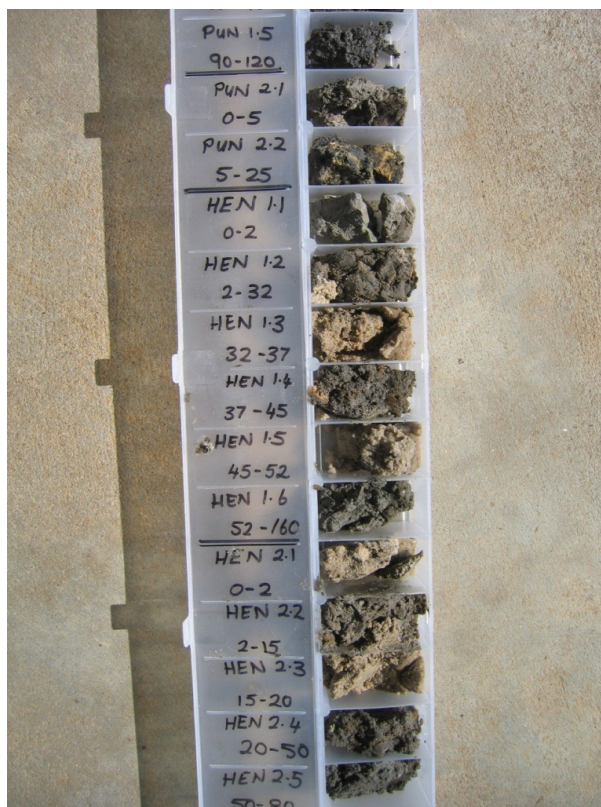
Figure 3–2. Example of a chip-tray sample showing the inside lid marked up adjacent to the soil sample collected to show soil morphology (photograph provided by G Grealish).
