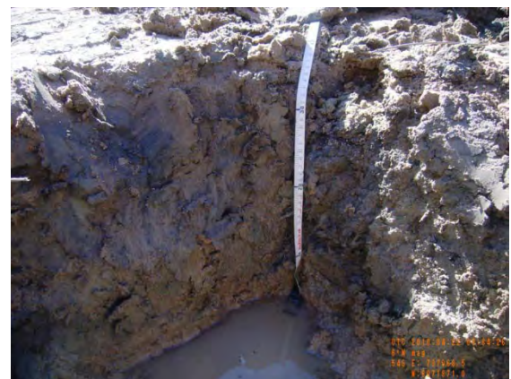
Figure 8 – Photographs of site 40304_6, showing the surface condition and the soil profile of dark greyish brown loose and very weak clayey sand.
