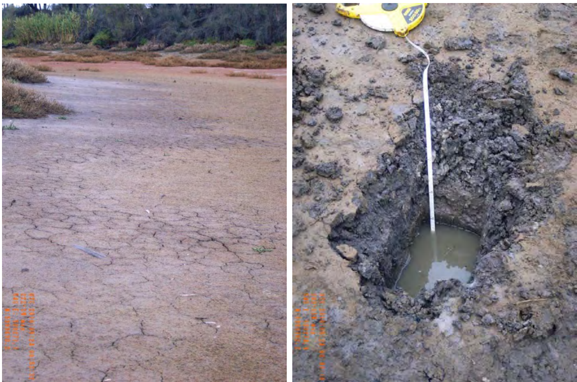
Figure 4 – Photographs of site 40855_2, showing the surface condition and the soil profile of very weak, very dark grey silty clay loam overlying firm, greyish brown, silty clayey sand.
