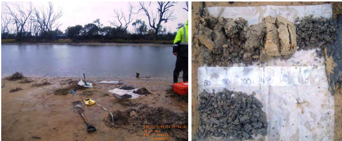
Figure 6 – Photographs of site 40855_4, showing the surface condition and the laid out soil profile of very weak, dark greyish brown sandy clay loam overlying weak, very dark grey, loamy sand and clay loam.
