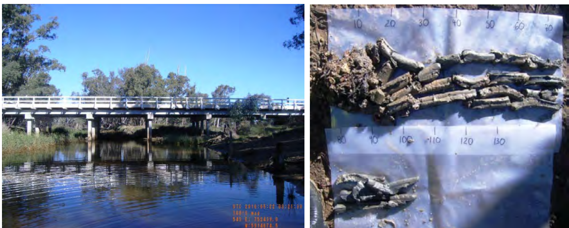
Figure 5 – Photographs of site 40860_3, showing the water surface (water column of 45cm), and the laid out soil profile of loose to weak, brown silty loam and clay overlying soft, very dark bluish grey silty clay loam.
