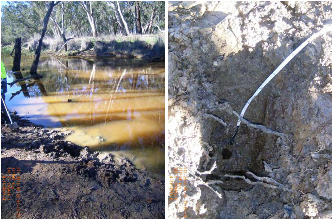
Figure 6 – Photographs of site 40860_4, showing the surface condition and the soil profile of soft, dark brown silty clay loam overlying very weak, dark greyish brown clay.
