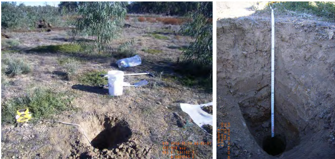
Figure 6 – Photographs of site 40590_4, showing the surface condition and the soil profile of strong, very dark greyish brown silty clay loam overlying very firm, dark greyish brown clay.
