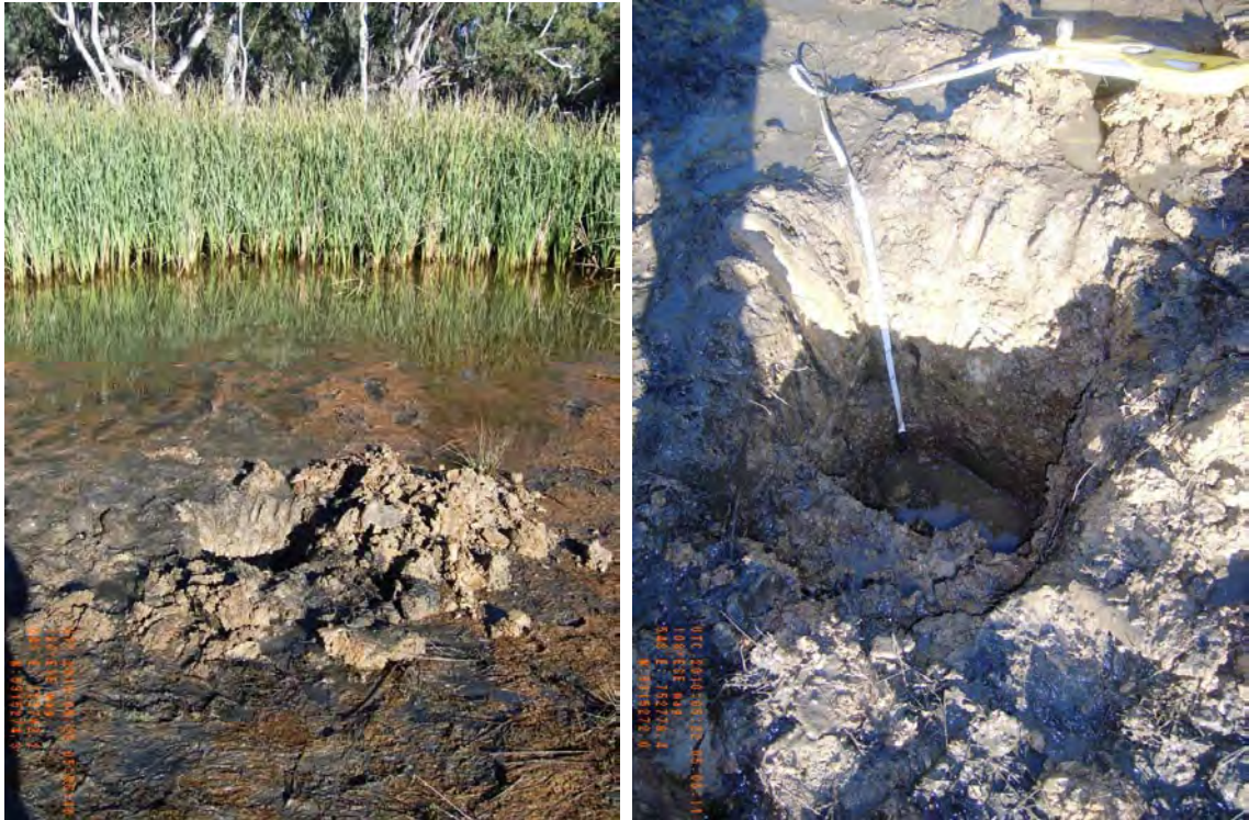
Figure 8 – Photographs of site 40861_2, showing the surface condition and the soil profile of very soft, yellowish brown clay loam and clay overlying very weak, very dark greyish brown silty clay loam.
