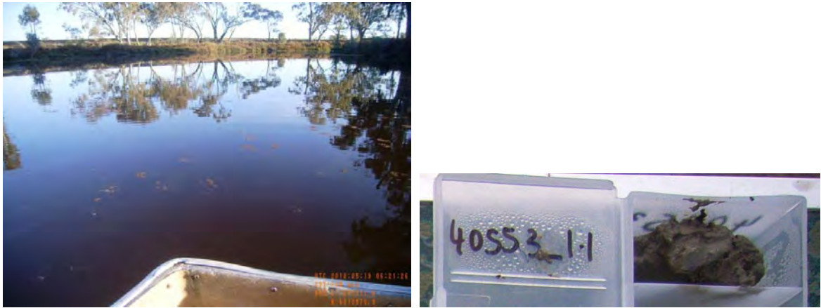
Figure 3 – Photographs of site 40553_1, showing the water surface (water column of 1.80m), and the chip tray soil profile of dark grey, very soft, wet, clay.
