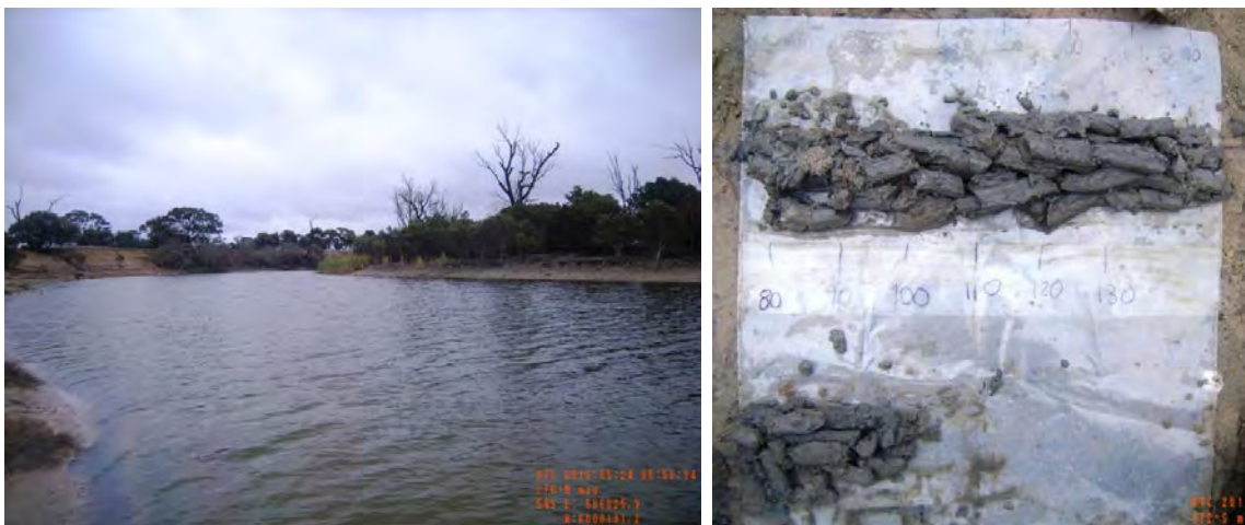
Figure 7 – Photographs of site 40855_5, showing the water surface (water column of 40cm), and the laid out soil profile of very weak, dark grey sandy loam overlying weak, dark grey to bluish grey sandy clay loam.
