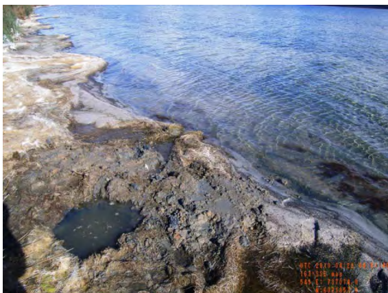
Figure 9 – Photographs of site 40304_7, showing the edge of water surface condition and the chip tray soil profile grey to dark grey soft clayey sand overlying reddish brown soft sandy clay.
