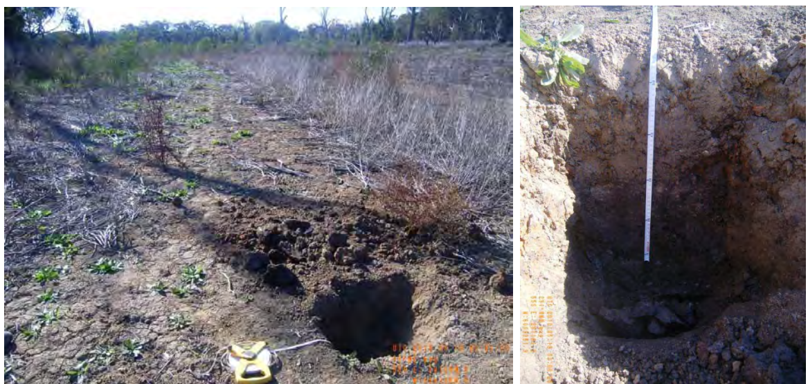
Figure 4 – Photographs of site 40590_2, showing the surface condition and the soil profile of strong, very dark greyish brown silty clay loam overlying very firm, dark greyish brown clay.
