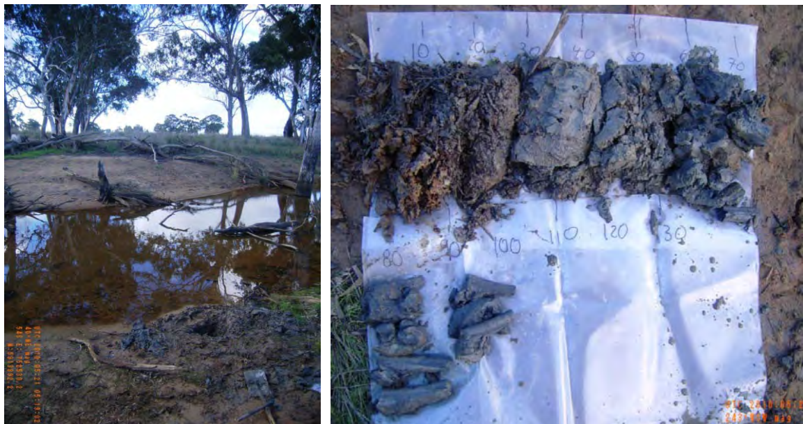
Figure 14 – Photographs of site 40863_2, showing the surface condition and the soil profile very soft, dark grey to dark brown clay loam overlying soft, dark greenish grey clay.
