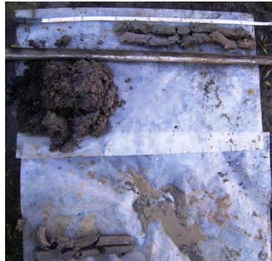
Figure 7 – Photographs of site 40416_5, showing the water logged surface (water column of 8cm) and the laid out soil profile of dark greyish brown, soft, loam overlying dark grey, very soft, clay.
