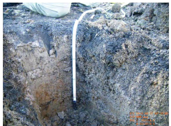
Figure 9 – Photographs of site 40416_7, showing the surface condition and soil profile of greyish brown, very weak, clay overlying dark greyish brown, weak, clay.
