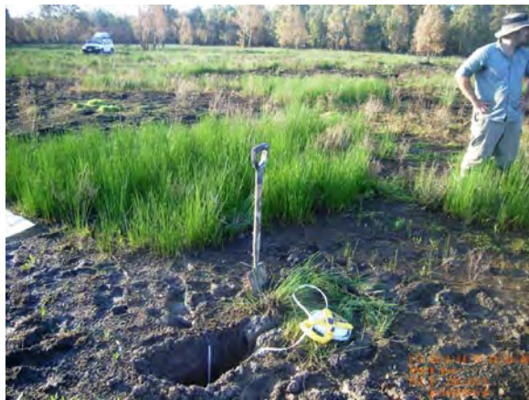
Figure 8 – Photographs of site 40416_6, showing the surface condition and soil profile of dark greyish brown, soft, clay overlying dark greyish brown, very soft, clay.
