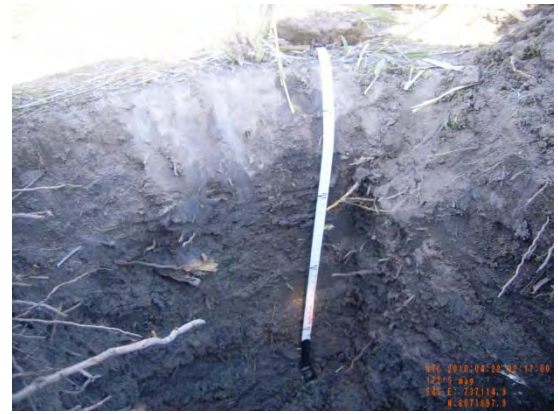
Figure 7 – Photographs of site 40304_5, showing the surface condition and the soil profile of dark greyish brown loose loamy sand overlying reddish brown very weak clayey sand.
