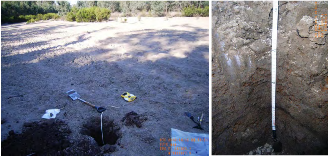
Figure 9 – Photographs of site 40383_7, showing the stream channel surface condition and the shallow soil profile reddish brown, strong, silty clay loam and clay.
