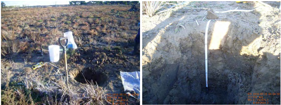
Figure 6 – Photographs of site 40486_4, showing the surface condition and the soil profile of weak, brown and dark brown clay loam overlying very firm, dark greyish brown clay loam sandy.
