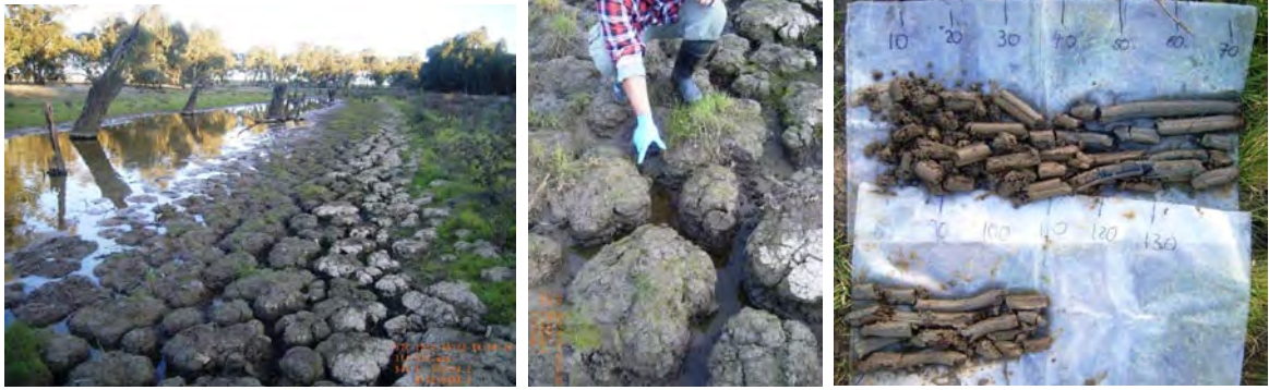
Figure 10 – Photographs of site 40861_4, showing the surface condition and the soil profile of very weak, brown silty clay loam overlying weak, brown some grey brown clay.
