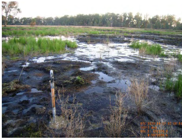
Figure 7 – Photographs of site 40416_5, showing the water logged surface (water column of 8cm) and the laid out soil profile of dark greyish brown, soft, loam overlying dark grey, very soft, clay.
