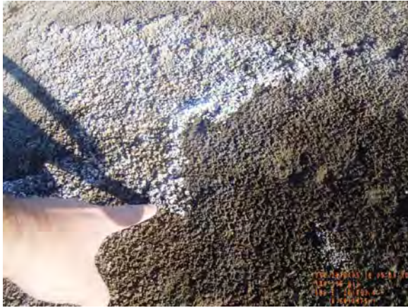
Figure 5 – Photographs of site 40486_3, showing the surface condition, surface salt crust and the soil profile of loose salt crust on surface, then weak, brown clay loam overlying very firm, dark grey clay.
