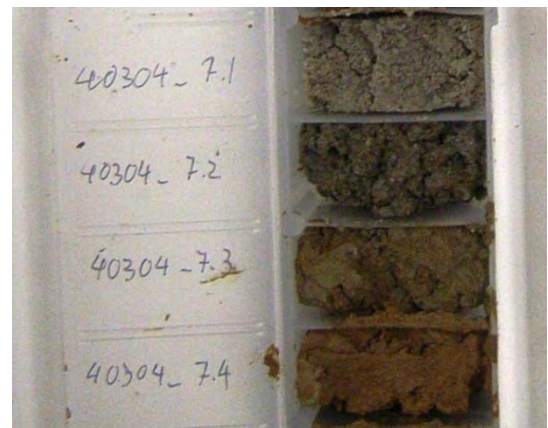
Figure 9 – Photographs of site 40304_7, showing the edge of water surface condition and the chip tray soil profile grey to dark grey soft clayey sand overlying reddish brown soft sandy clay.
