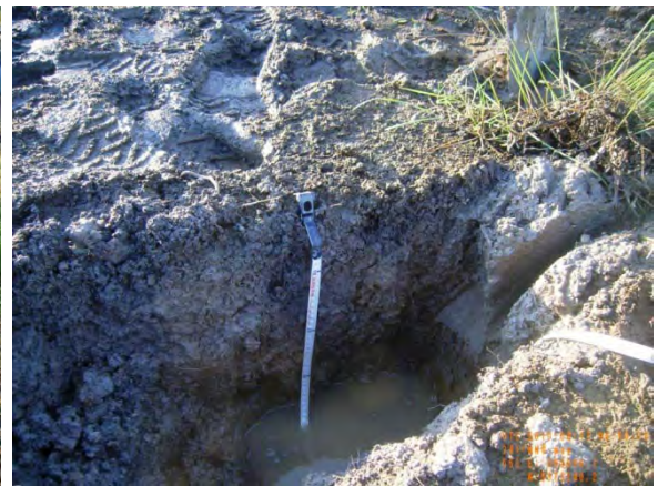
Figure 8 – Photographs of site 40416_6, showing the surface condition and soil profile of dark greyish brown, soft, clay overlying dark greyish brown, very soft, clay.
