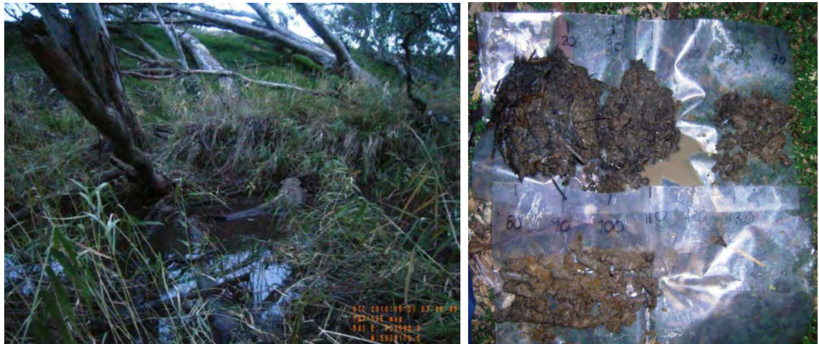
Figure 3 – Photographs of site 40851_1, showing the water surface (water column of 50cm), and the laid out soil profile of very soft, dark yellowish brown clay loam overlying very weak, dark greyish brown silty and sandy clay loam.
