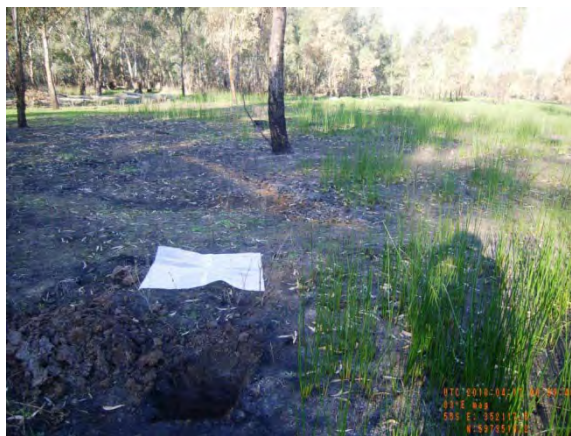
Figure 9 – Photographs of site 40416_7, showing the surface condition and soil profile of greyish brown, very weak, clay overlying dark greyish brown, weak, clay.
