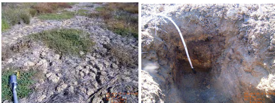
Figure 4 – Photographs of site 40486_2, showing the surface condition and the soil profile of weak, dark greyish brown clay loam overlying very firm, dark greyish brown clay.
