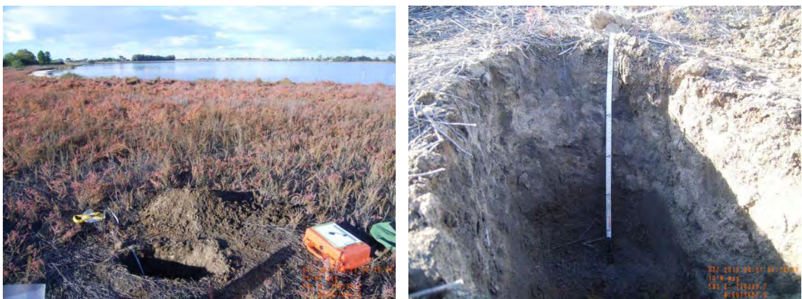
Figure 5 – Photographs of site 40304_3, showing the surface condition and the soil profile of grey loose loamy sand overlying reddish brown very weak clayey sand.
