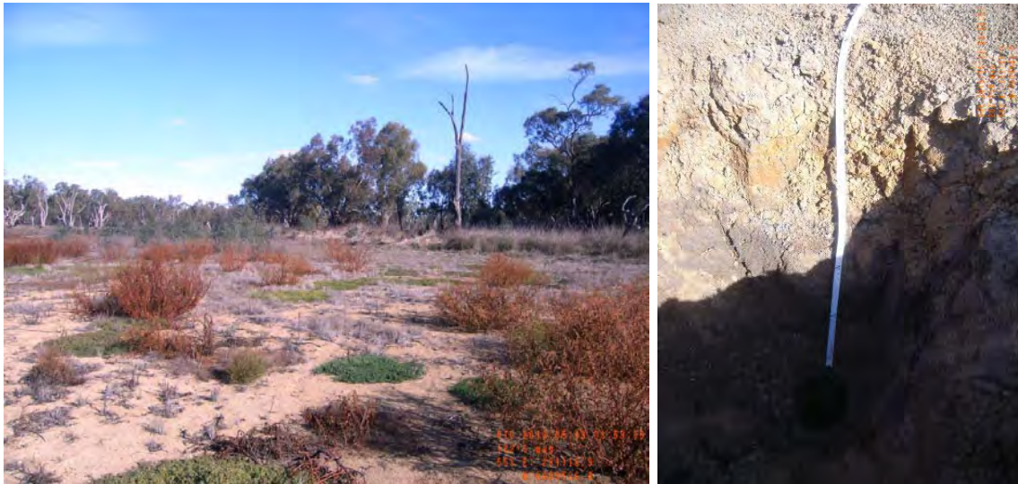
Figure 5 – Photographs of site 40590_3, showing the surface condition and the soil profile of strong, dark greyish brown clay overlying very firm, brown clay.
