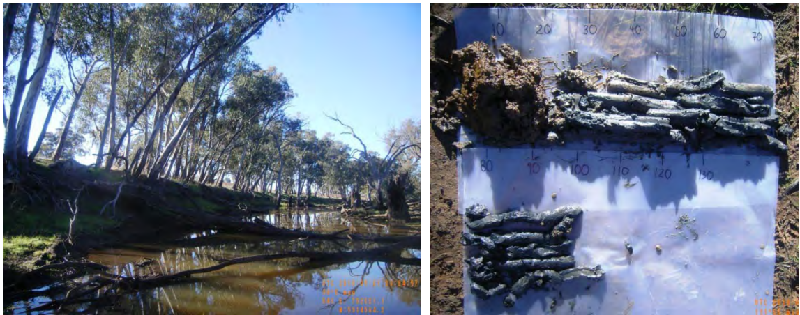
Figure 3 – Photographs of site 40860_1, showing the water surface (water column of 40cm), and the laid out soil profile of soft, dark yellowish brown silty clay loam overlying very weak, black silty clay loam.
