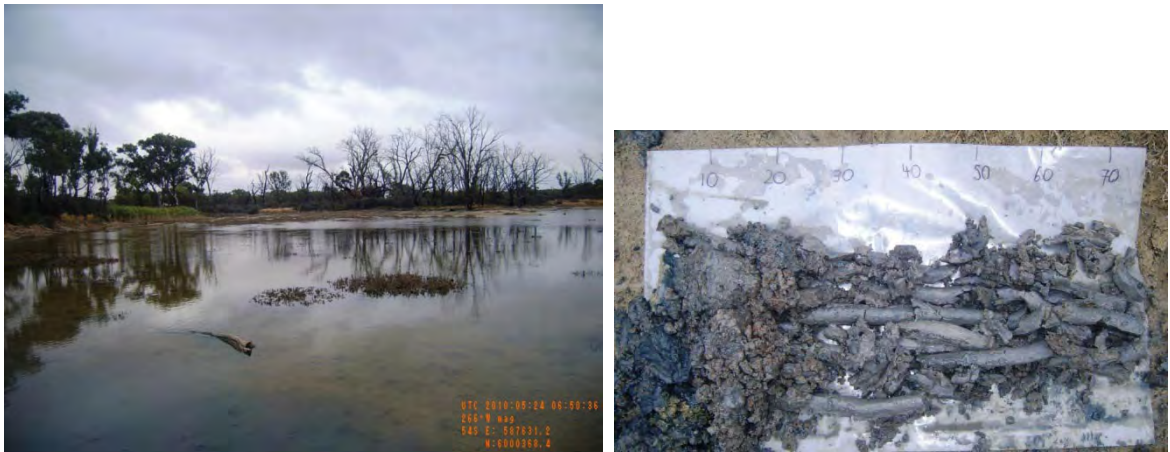
Figure 9 – Photographs of site 40855_7, showing the water surface (water column of 18cm), and the laid out soil profile of very soft, dark grey silty loam overlying weak, dark grey silty clay loam.
