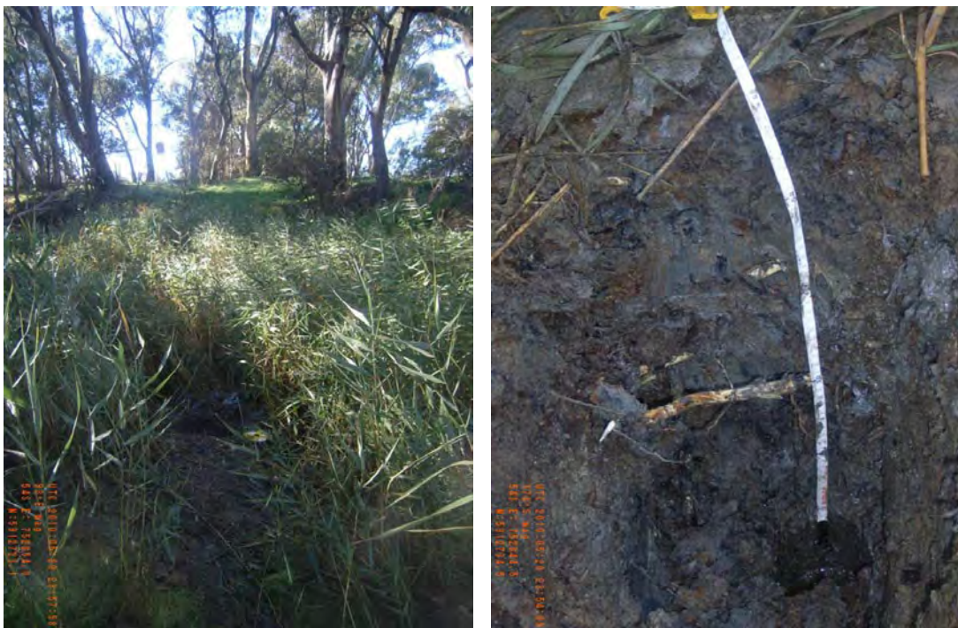
Figure 12 – Photographs of site 40862_2, showing the surface condition and the soil profile of very dark brown sandy loam overlying soft, bluish black silty clay loam.
