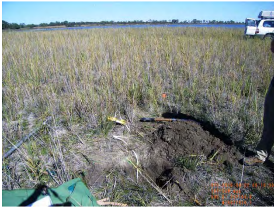
Figure 7 – Photographs of site 40304_5, showing the surface condition and the soil profile of dark greyish brown loose loamy sand overlying reddish brown very weak clayey sand.
